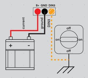
To detect this situation, the tracker needs an additional connection (DIN3 - orange/white or DIN4 - purple) to the chassis. This input can detect invalid signals and will allow the cloud platform to filter other invalid inputs as well. Make sure you enable input filtering in the cloud platform on digital input 3/4 when this feature is needed.
