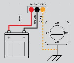
To detect this situation, the tracker needs an additional connection (DIN3 - orange/white or DIN4 - purple) to the chassis. This input can detect invalid signals and will allow the cloud platform to filter other invalid inputs as well. Make sure you enable input filtering in the cloud platform on digital input 3/4 when this feature is needed.
