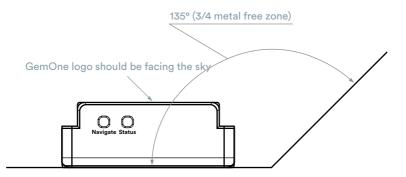
It is not important in which direction the tracker is installed. The most important instruction is that the GSM and GNSS antenna have a good open view.
