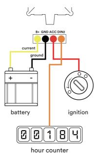
B+, GND and ACC (DIN1) are mandatory for every installation.
