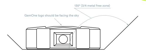
It is not important in which direction the tracker is installed. The most important instruction is that the GSM and GNSS antenna have a good open view.
