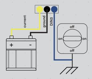
To detect this situation, the tracker needs an additional connection (DIN3 - blue) to the chassis. This input can detect invalid signals and will allow the cloud platform to filter other invalid inputs as well. Make sure you enable input filtering in the cloud platform on digital input 3 when this feature is needed.
